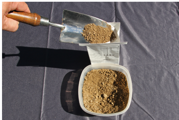
Figure 11: Take about one pint of the composite sample to be sent for testing.
