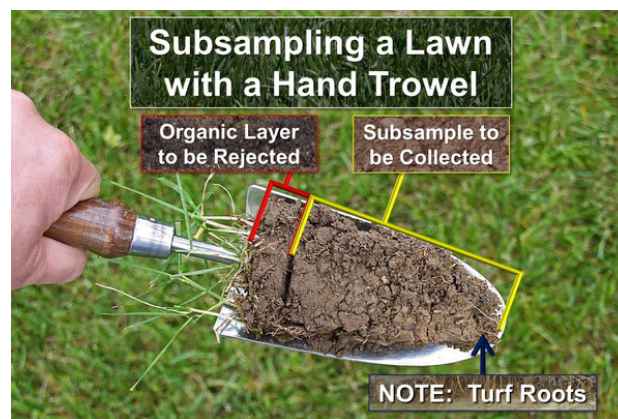
Figure 6: Using a hand trowel for soil sampling. Photo by Joe Boggs, Ohio State University Extension.
