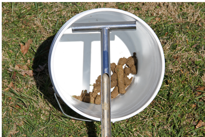
Figure 7: Soil samples should be collected in a clean plastic bucket. Photo by Joe Boggs, Ohio State University Extension.
